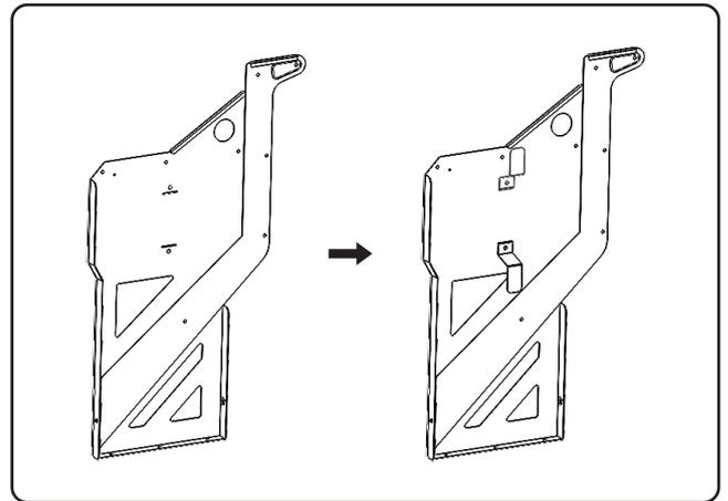
**3** Find the right side panel, the two brackets, and the right outer panel. First, position the right outer panel onto the right side panel as shown in the diagram, and fasten it with screws. Then, attach the brackets using screws.
