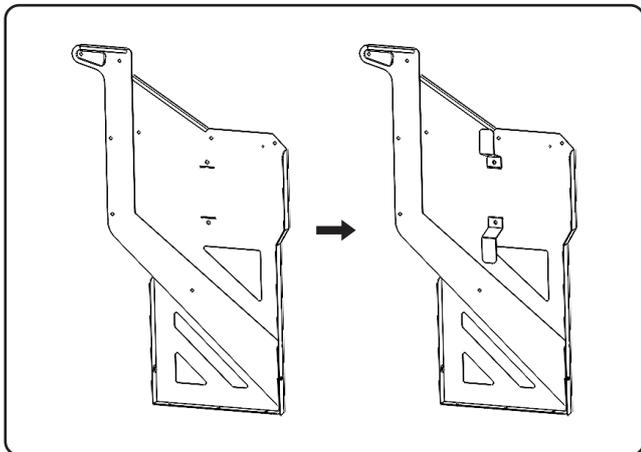
**4** Assemble the components from Steps 1, 2, and 3 together using screws.
