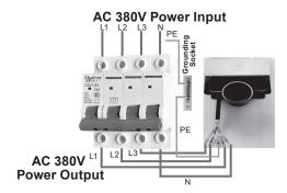
As shown in the diagram, connect the five wires at the input end of the charging station (L1 = Line 1, L2 = Line 2, L3 = Line 3, N = Neutral, PE = Protective Earth) to the respective terminals on the circuit breaker. Then, connect the circuit breaker to the mains power supply.
