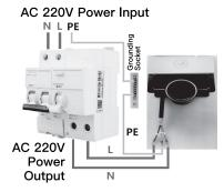
As shown in the diagram, connect the three wires at the input end of the charging station (L = Line, N = Neutral, PE = Protective Earth) to the respective terminals on the circuit breaker. Then, connect the circuit breaker to the mains power supply.
