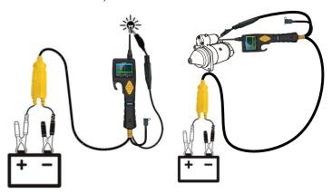
If the probe circuit breaker tripped, it means the probe is overloaded. This could happened by the following reasons:
