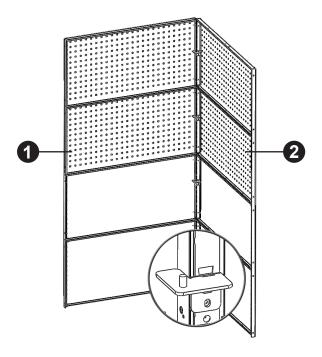
Step 2: Insert the 4 [3] Shelf Beams into their respective positions from bottom to top.
